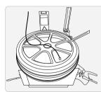
Dismantle the valve core with valve core removal tool. Then inflate the tire to the nominal value according to the tire data plate the vehicle. Install the valve core and screw the valve cap.
