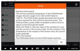
Figure 5-14 Sample DTC Help Screen
