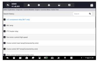
Figure 5-27 Sample Active Test Screen
