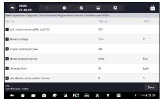
Figure 5-13 Sample Freeze Frame Screen
