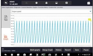
Figure 5-21 Sample PID Graph Screen
